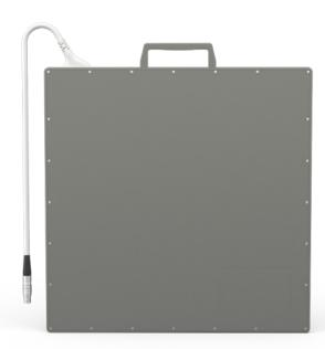
**X-Panel 4343a PSI** is a portable type and low noise X-ray flat panel detector optimized for industrial non-destructive testing (NDT) and digital radiography (DR) applications. It is based on amorphous silicon (a-Si) technology that features a high dynamic range and a long lifetime among other benefits.
